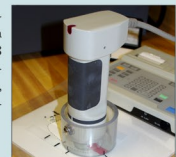
Fig. 7. Minolta CR-300 Chroma Meter, measuring platform, test sample, and jig
